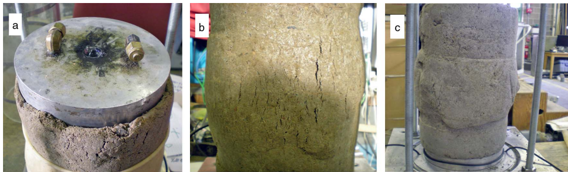
Fig. 5. (a) Expansion of RSG mixed with 15% by weight of CKD after 28-day curing before testing; (b) bulging of the RSG mixed with 15% CKD after bench-scale resilient modulus testing; and (c) shear failure in RPM mixed with 15% of CKD after bench-scale resilient modulus testing (specimen diameter is 150 mm)
